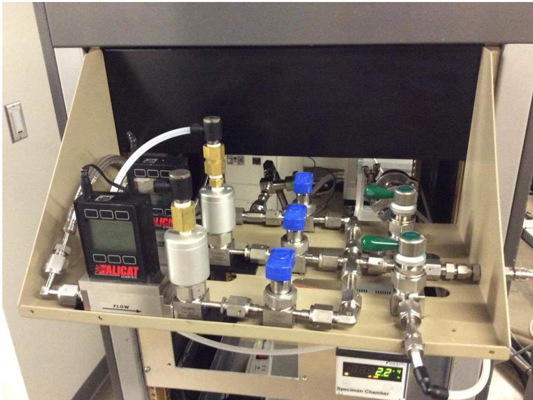
The Gas Delivery System for the Hitachi H-9500 E-TEM is designed to delivery up to 2 process gasses controlled in parallel and one evaporation liquid source. It has dry pump rough vacuum and built in nitrogen purge for fast process gas switching.
